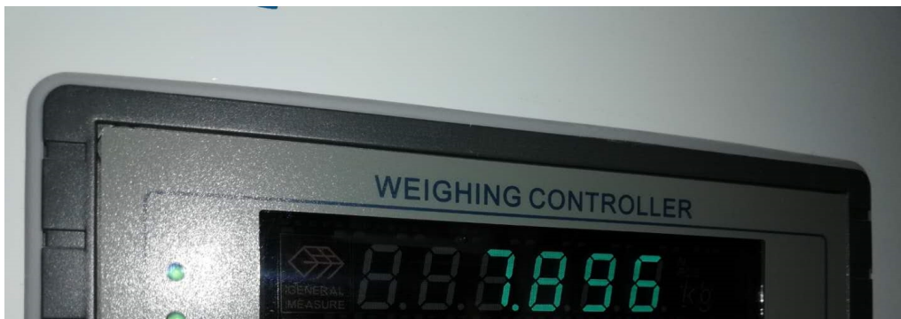
Calibration display sequence - test-weight entry
