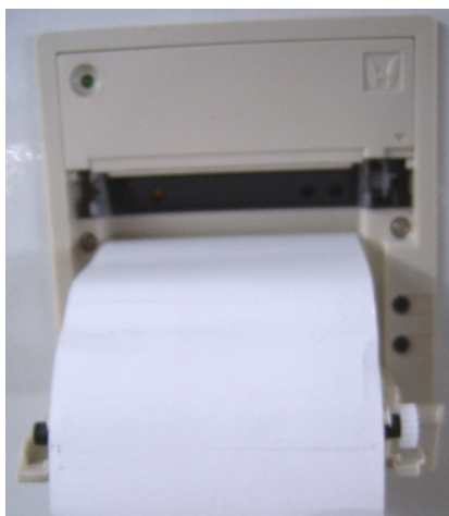
Printer cover and paper-roll arrangement
